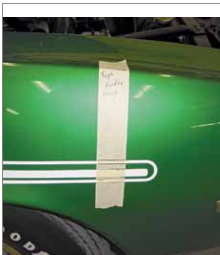
Before the stripes were removed, measurements and notes were taken to ensure accurate replacement.
