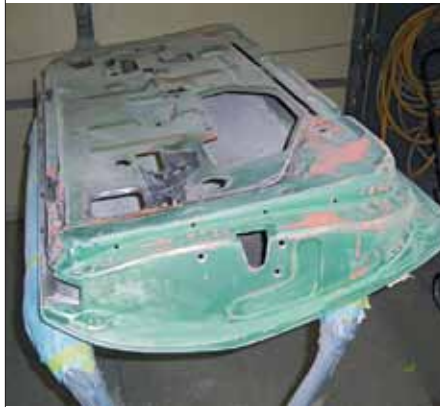
Orange paint was discovered, so this door was media blasted rather than chemical stripped in order to get in all of the nooks and crannies.
