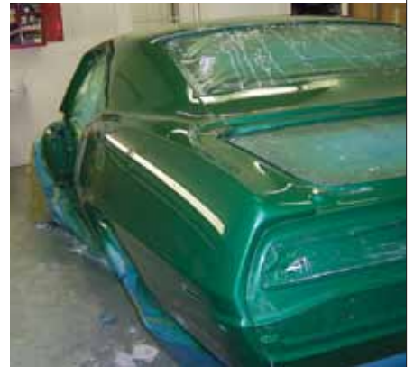
Fresh basecoat/clearcoat urethane paint was applied. The Rally Green color was replicated using a spot concealed under a trunk decal.
