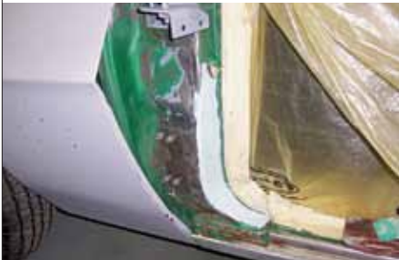
Some repair work was needed in the car's cowl, and the driver's door was orange under the paint. Otherwise, it was as new.
