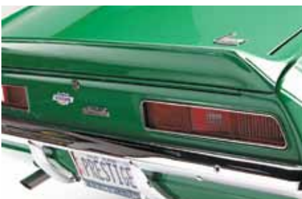
The offset emblems on the rear were installed in place of the bowtie emblem by drilling just two holes and using two existing ones.
