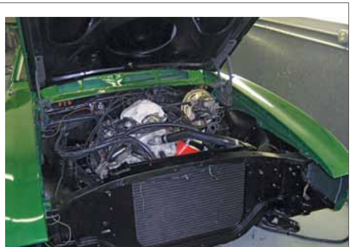
Fresh paint on the inner fenders and radiator support, new tower hose clamps and some new, correct fasteners make the car like-new again.
