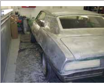
The car had received one repaint and was stripped bare with a combination of chemical stripping and media blasting.
